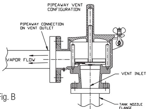
A pipe-away device (Fig. B) usually includes two mounting connections. One connection mounts the vent to the tank (inlet) and the other connection (outlet) is usually joined to a pipe that directs vapors to some location for further processing.
