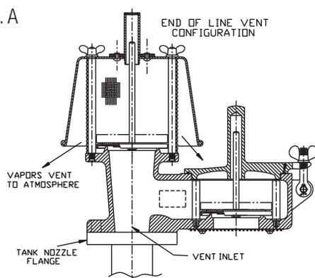
In an end-of-line device (Fig. A), a single flanged / threaded connection (inlet) is included as a part of the housing. The vent is mounted to the tank's nozzle and any flow of vapor/air into or out of the tank is communicated to the atmosphere.
