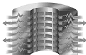
Figure 14.15.1 Tiger-Tooth Vent Flow Pattern
