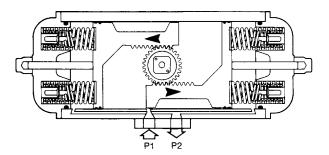
Exhausting the air pressure from Port 1 allows stored energy of the springs to drive pistons inward, turning the pinion clockwise. Air volume on outside of pistons vents through Port 2.
