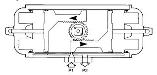
Applying air pressure to Port 2 drives the pistons inward, which turns the pinion clockwise as the air volume on the inside of the pistons exhausts through Port 1.
