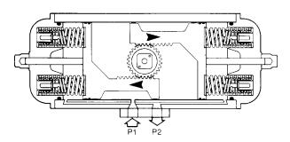
Exhausting the air pressure from Port 1 allows stored energy of the springs to drive pistons inward, turning the pinion counterclockwise. Air volume on outside of pistons vents through Port 2.
