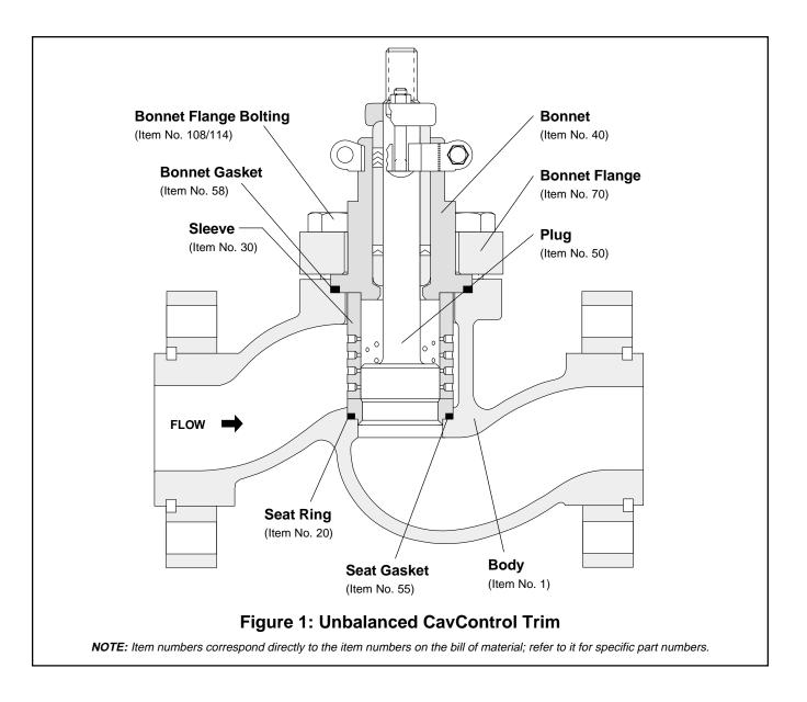
3. If the pressure-balanced sleeve binds with the plug, carefully lift the sleeve out with the actuator/plug assembly. Place several sturdy, soft supports (preferably wood) underneath the sleeve after it clears the body. Lower the actuator/plug assembly until the sleeve and the supports are resting on top of the body.
