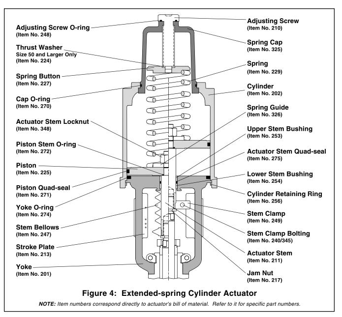
movement into the bore. For *air-to-extend* configurations, repeat this process without the thrust washers or springs. Once the piston is installed and leveled, center the spring on the piston.
