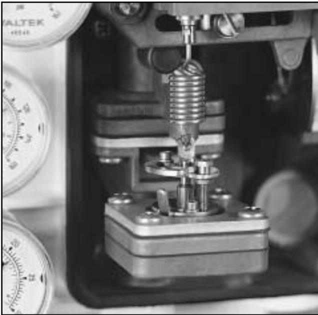
**Figure 7: Close-up of Gain Adjustment**
